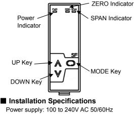
Power supply: 100 to 240V AC 50/60Hz 24V AC/DC 50/60Hz Allowable voltage range: 85 to 264V AC 20 to 28V AC/DC Power consumption: Approx. 6VA
